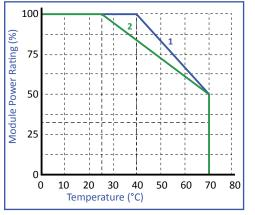
\* Module can deliver 95% of rated power at 25°C ambient.
